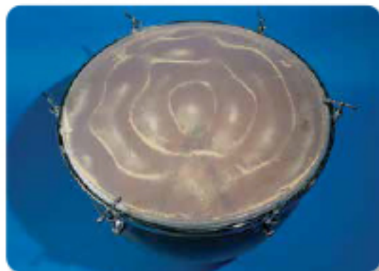
Sand sprinkled on a drum skin shows the waves formed when it vibrates.
